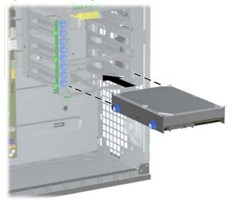
**Figure 5-26** Installing a Hard Drive into the Hard Drive Bay
